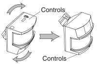
If the sensor pops out of the ball joint, loosen the clamp screw and push the sensor back into the ball joint. Tighten the clamp screw when done.
